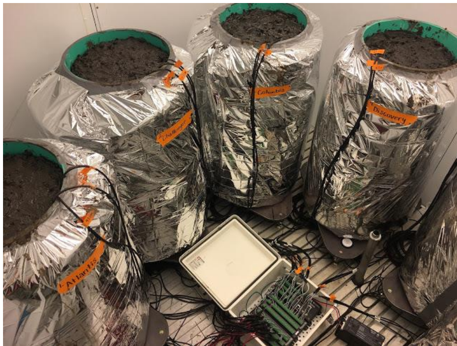
Figure 4-3: Six columns positioned around the data logger within the environmental chamber, at the beginning of the experiment.
