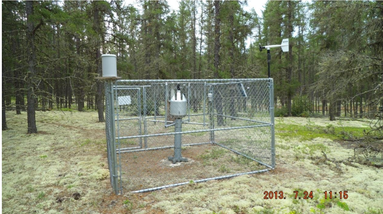
Figure 3.4 Geonor-T200B weighing gauge for measuring precipitation installed at the jack pine site
