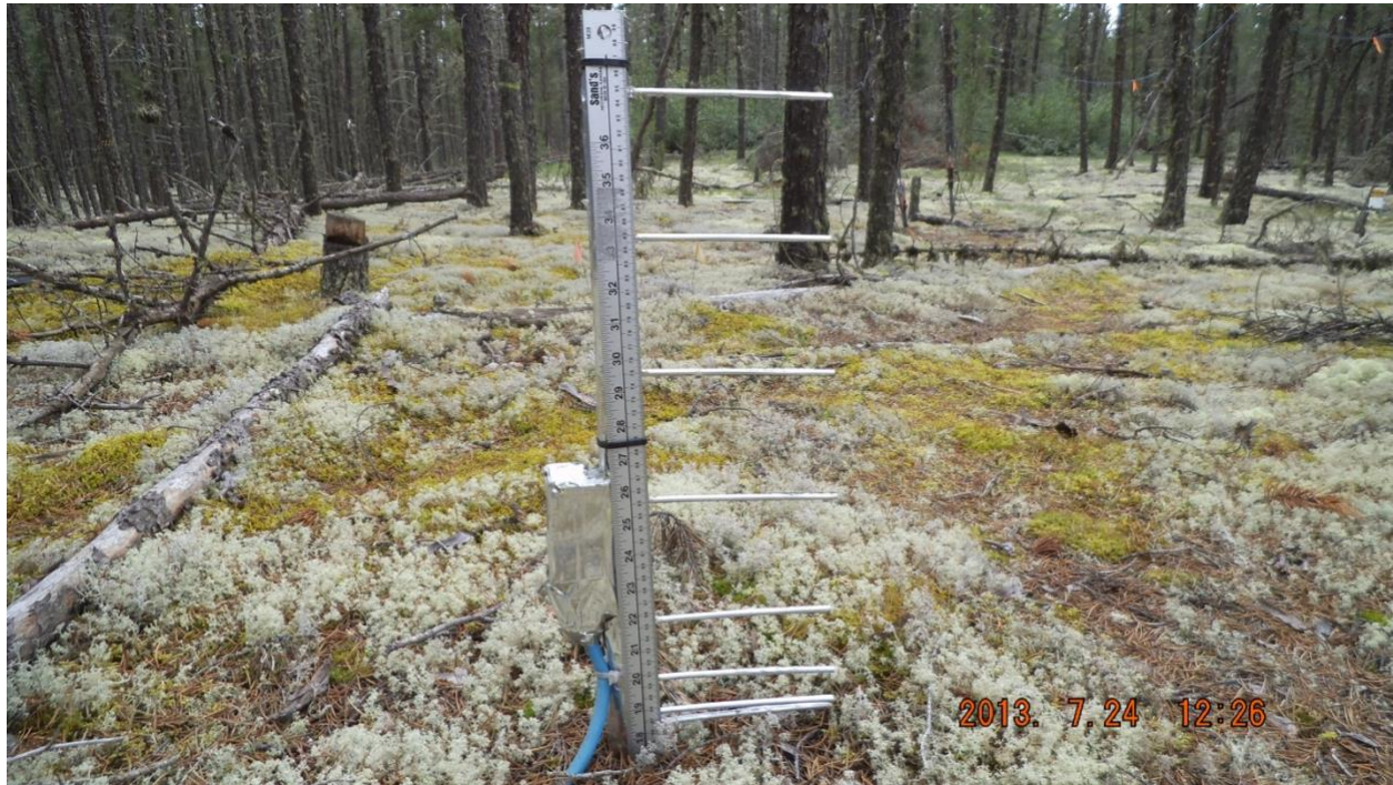
Figure 3.10 Snow temperature probes installed at site
