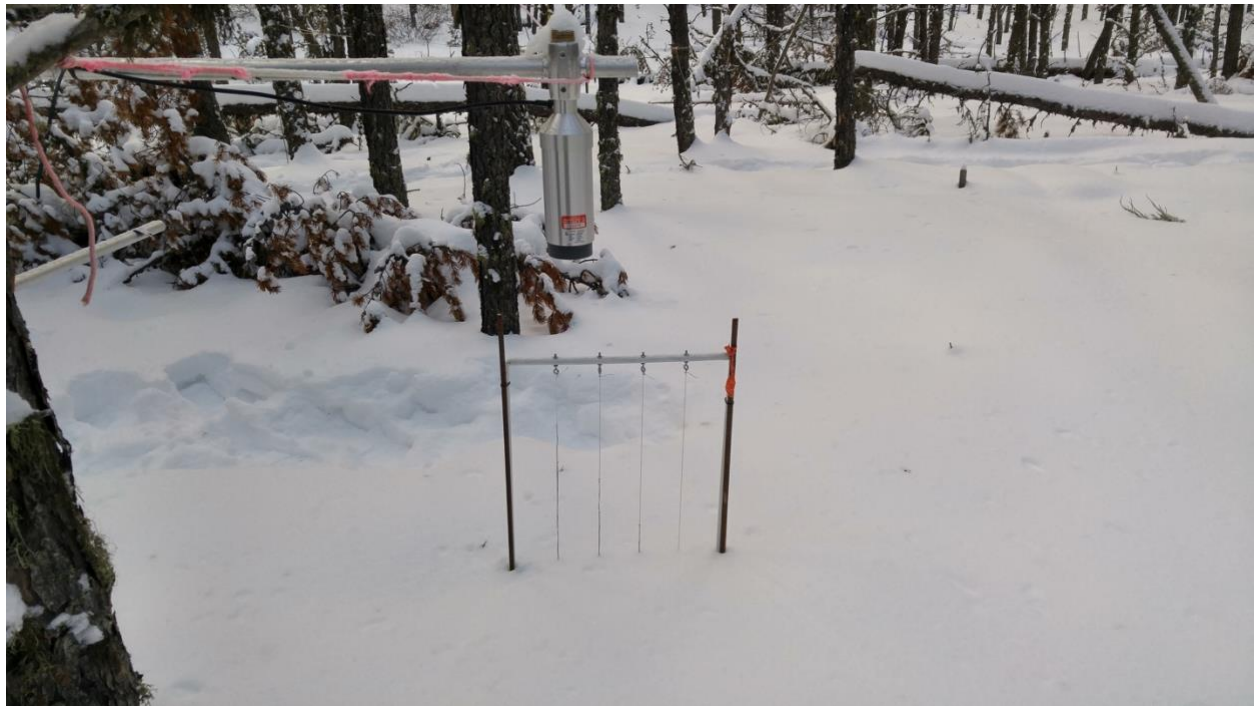
Figure 3.11 Snow harp for measuring snow temperature at every 5 cm depth, and SR-50 for measuring snow depth installed at the jack pine site
