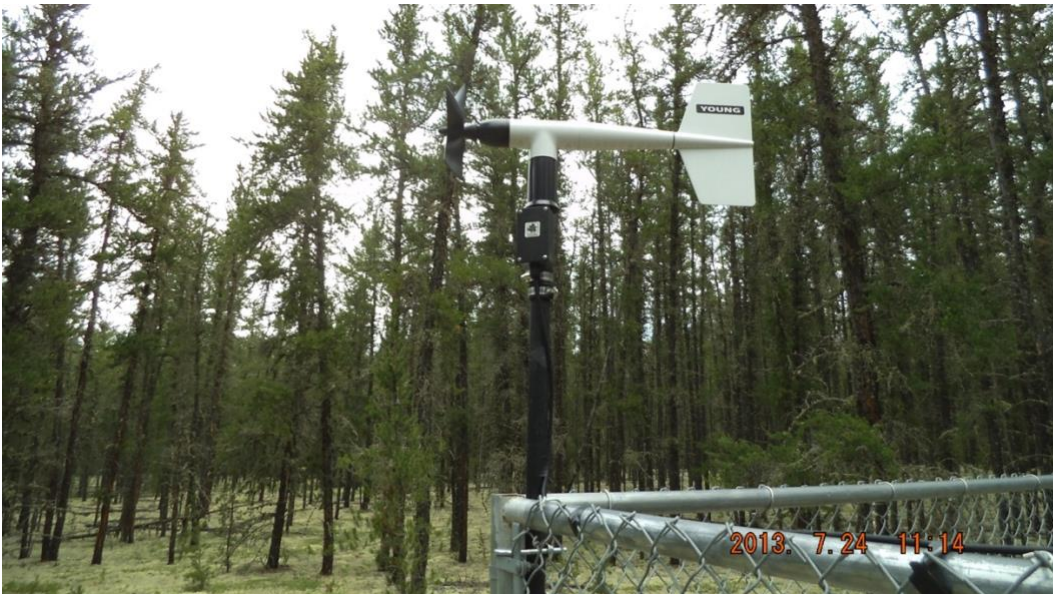
Figure 3.8 Sensors for measuring wind speed and direction
