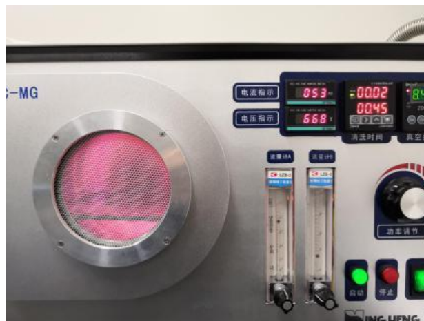
Fig. 5.6. The oxygen plasma applied to bond the PDMS with the glass.
