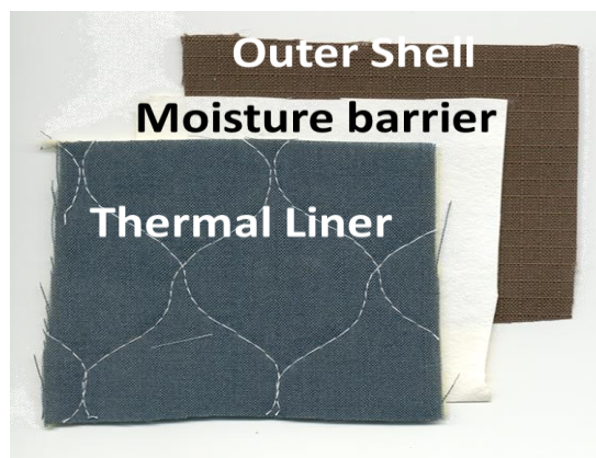
Figure 1.1: Basic layers of a complete firefighters' protective coat.
