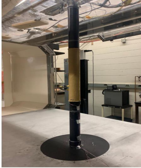
Figure 3.6: The 2D cylinder in the wind tunnel with PBI Max fabric wrapped around it (airflow is from left to right).
