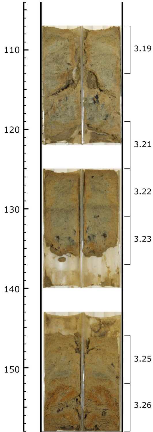
Figure 5.3: Sampling column 3 sediments. Subsamples are noted to the right of the column. Blank spaces correspond to bagged material from the end of the coring device. Samples 3.25 and 3.26 were shifted up to correspond to field measurements.
