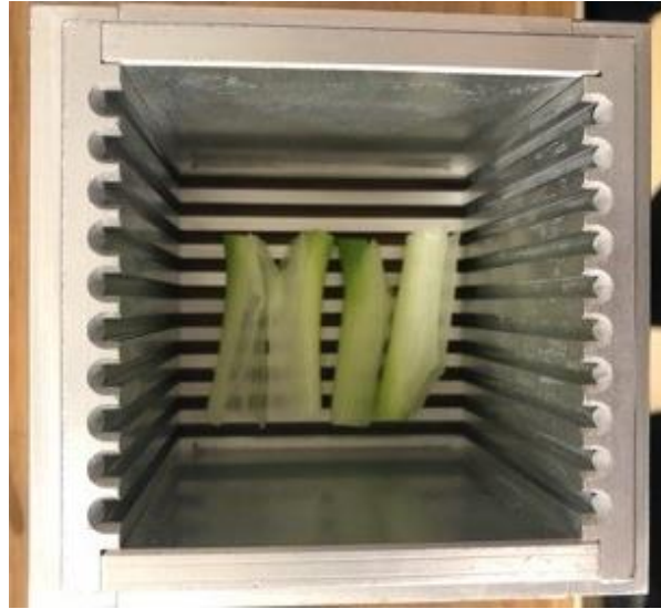
Figure A2 Placement of Allium fistulosum sheaths in texture analyzer cell
