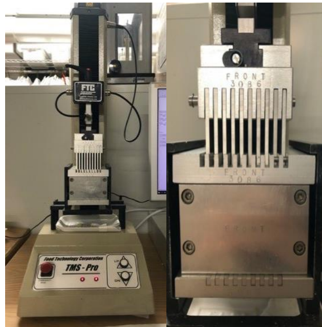
Figure A3 TMS-Pro texture analyzer with 10-blade Allo-Kramer shearing compression cell
