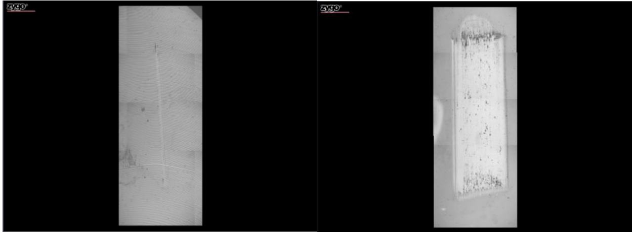
Figure 4.14. Optical image of wear track Nb-DLC films with 17.4 at. % Nb (left) and 24.0 at. % Nb (right)
