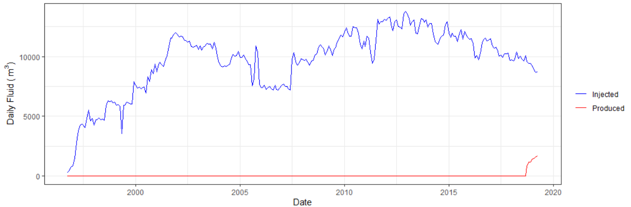
Figure 6-3: Combined daily production (red) and injection (blue) rates (m 3 ) in the Aqtesolv model area for the Mannville Group
