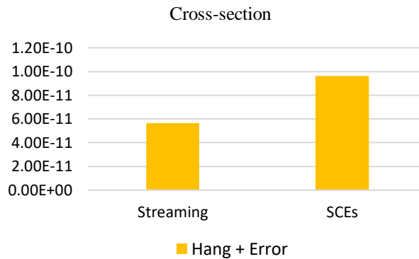
Figure 5.2 Cross-sections of total failures for each design
