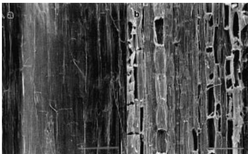
Figure 2.10. Scanning electron micrographs of barley straw, (a) untreated or (b) incubated in a 1:10 dilution of concentrated enzyme product containing cellulases and xylanases. Adapted from Bedford and Partridge (2010).
