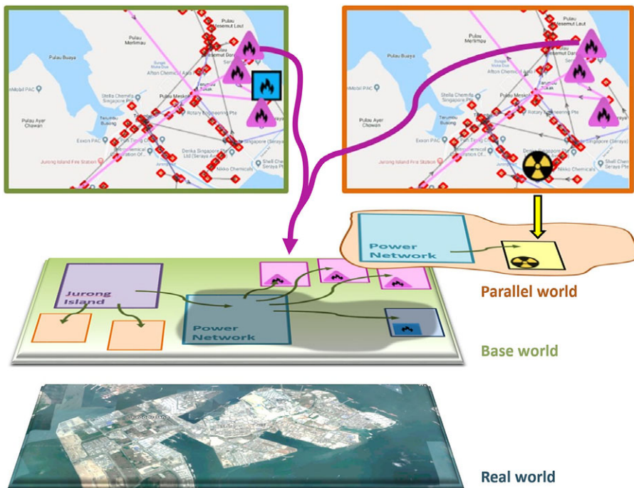
Figure 5. Parallel world concept for what-if scenario analysis. The panels at the top illustrate the electrical network from the real world (left) and an optimized network that is subject to a carbon tax (right). The network from the real world is described in the base world. The modifications to the network in the parallel world are described in a scenario-specific part of the knowledge graph. The pink triangles denote natural gas generators that are present in both the base world and the parallel world. The blue square denotes an oil generator that is only present in the base world. The radiation symbol denotes a small modular nuclear reactor that is only present in the parallel world. Adapted from Eibeck et al. (2020).
