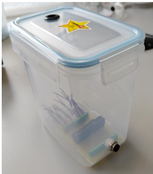
Figure 2.14 Hypoxia chamber for gas equilibration.
