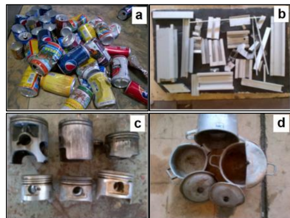
Figure 2. Recycled aluminum alloy: (a) used cans, (b) used profiles, (c) used engine pistons, and (d) used pans [27].
