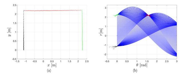
Figure 6. (a) Measurement data collected by 2D laser scanner Sick LMS 500, (b)  $r - \theta$  plane of (a) measurement data
