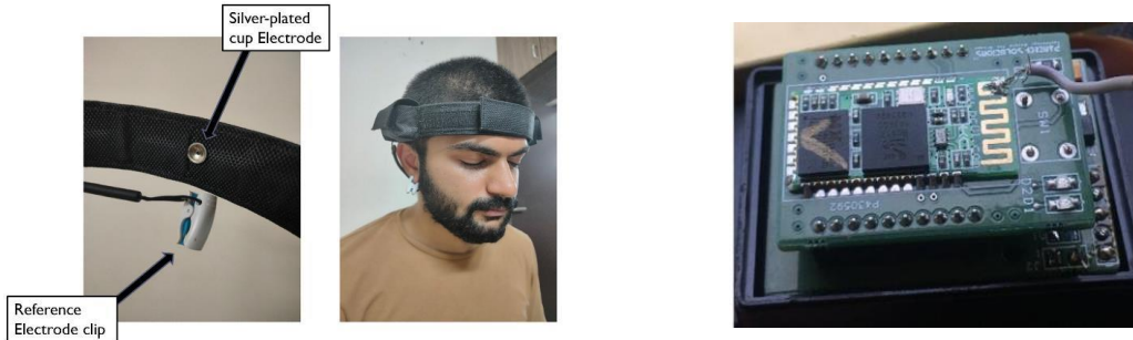
Figure. 13(a). Demonstration of the electrodes of the headwear and its proper placement on the head (b) ThinkGear ASIC Module integrated with a Bluetooth module
