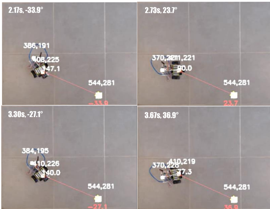
Figure 4.2 - Rover attempts to orient using overhead images to obtain heading error. 1). Heading error at 2.17s is -33.9°. 2). Heading error at 2.73s is 23.7°. 3). Heading error at 3.30s is -27.1°. 4). Heading error at 3.67s is 36.9°.
