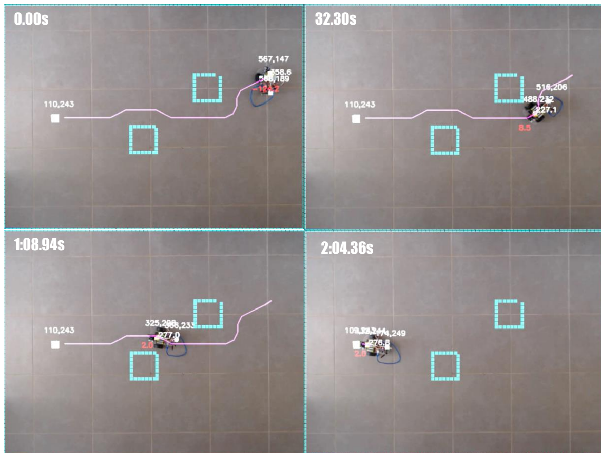
Figure 4.6 - The system using the potential field algorithm to navigate through a course of smaller obstacles. Four frames are shown at times 0.00s, 32.30s, 1:08.94s and 2:04.36s.
