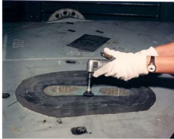
Figure 2-10: USN manual scarf machining (Baker 2006).
