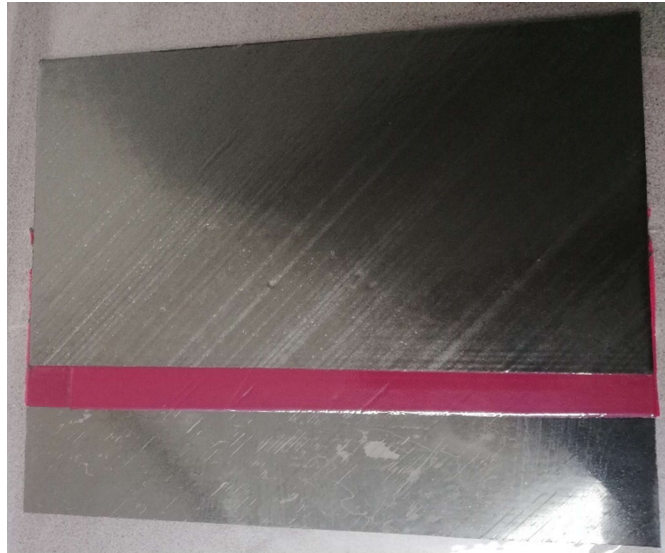
Figure 4-8: Initial adhesive overlap, which was reconsidered after pressure mapping.
