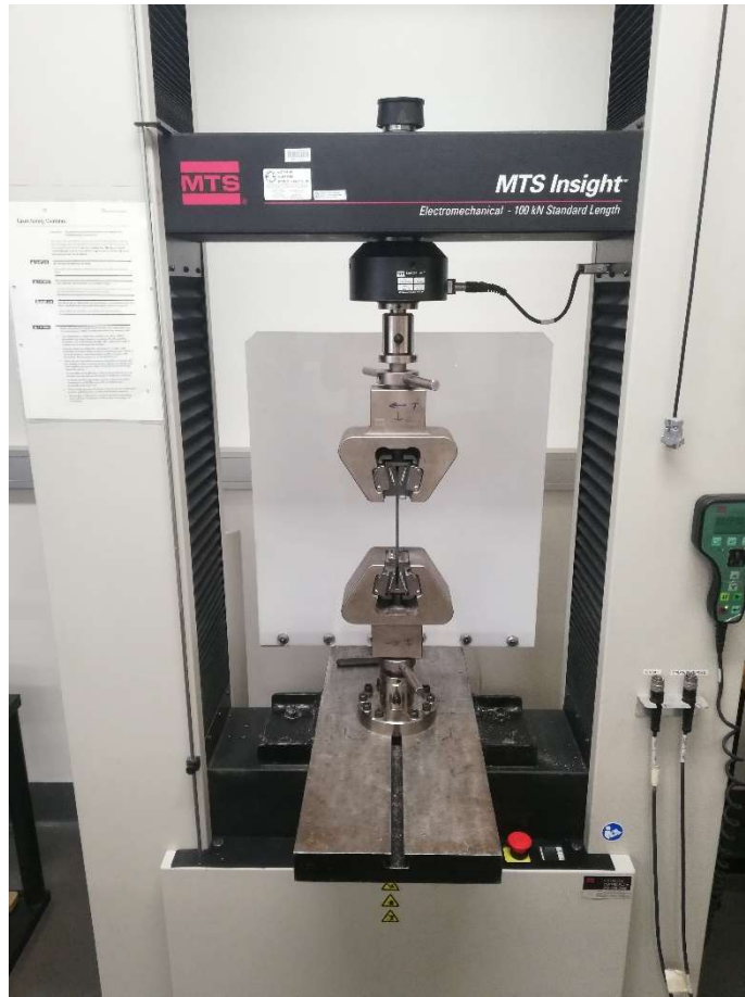
Figure 4-10: MTS Insight 100kN test rig w/ specimen.
