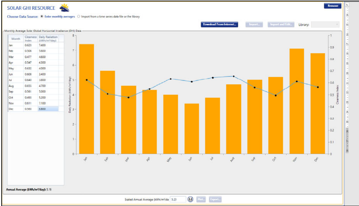
Figure 26: Solar GHI resource for Brisbane
