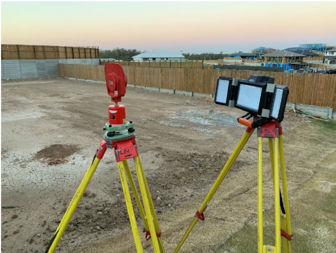
Figure 4.5, Experiment 5 – Flashlight Setup Used to Aid Low Light Observations.
