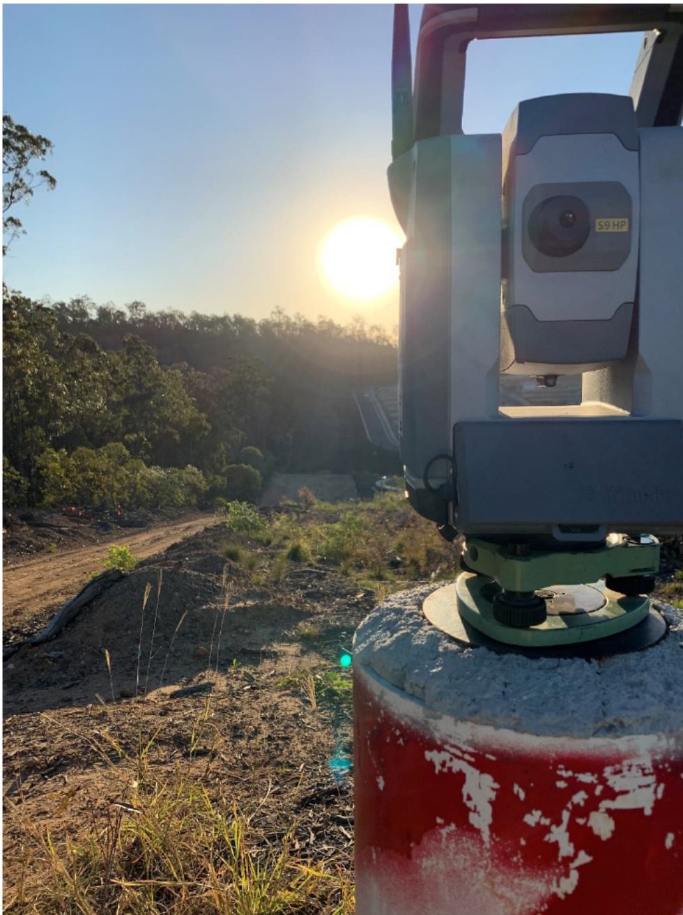
Figure 4.6, Experiment 6 – Sunlight Shinning Directly into Instrument
