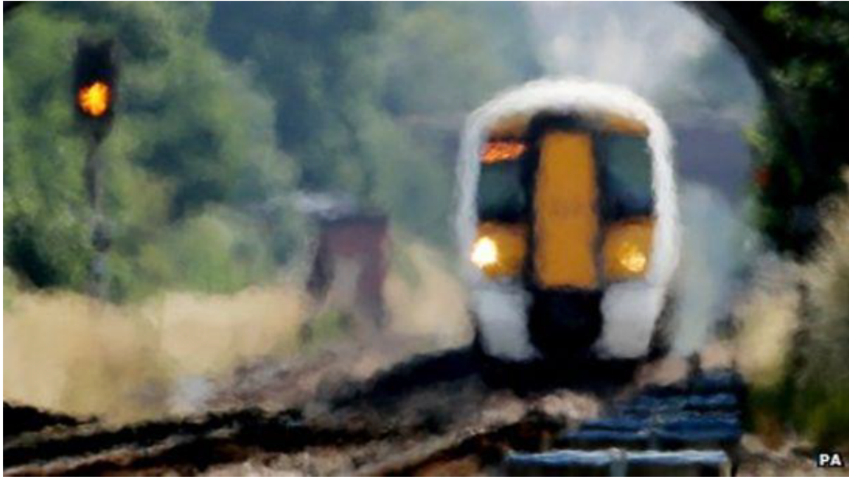
Figure 2.7, Example of the Effect of Heat Shimmer – sourced: https://www.bbc.com/news/magazine-23341698
