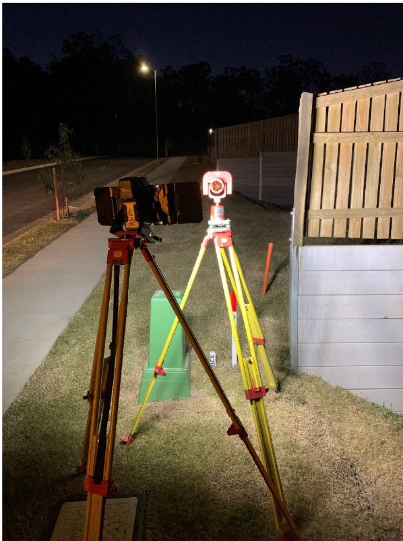
Figure 4.7, Experiment 7 – Flashlight Setup Being Used to Aid in Low Light Observations
