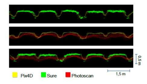
Figure 3: Cross section of 3D point clouds of crop surface computed with software packages Pix4D, Sure, Photoscan (Grenzdörffer 2014)
