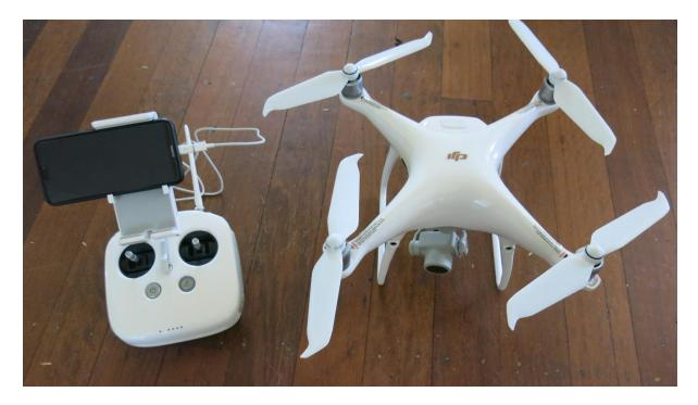
Figure 21: DJI Phantom 4 Pro V2.0 quadcopter UAV and controller with smartphone connected by usb cable
