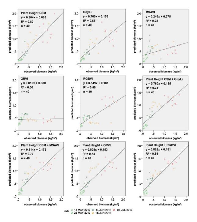
Figure 16: Barley biomass scatter plots and regression functions for predictions made using various linear regression and MLR models (Bendig et al. 2015)
