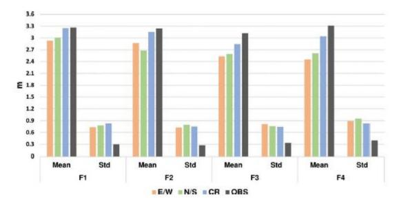
*Figure 6: Histogram showing mean and standard deviation of each approach for measuring height (E/W, N/S, combined E/W & N/S (CR) and Observed) for four test fields (De Souza et al. 2017)*
