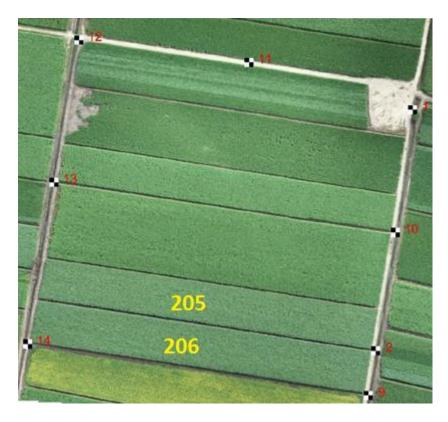
Figure 18: Aerial orthomosaic image of the site showing ground control points
