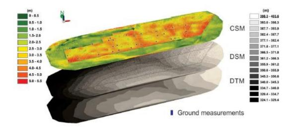
Figure 29: The CSM (shown in colour) represents crop height relative to terrain, whilst the DSM and DTM (shown in greyscale) represent elevations relative to a common datum (De Souza et al. 2017)
