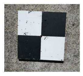
Figure 20: A target made from painted plywood
