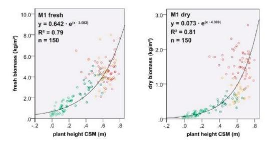
Figure 11: Yield prediction calibration models that exponential regression curves to describe relationship between CSMderived plant height and fresh biomass (left) and dried biomass (right) by Bendig et al. (2014)
