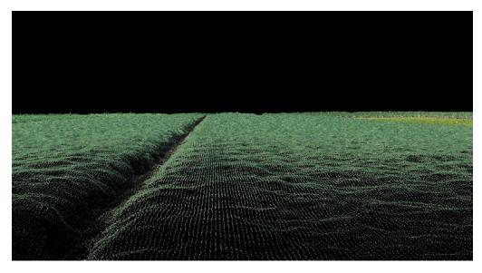
Figure 26: A low oblique close-up view of 3D Point cloud of surface of sugarcane. A drainage channel between the two subject fields is visible.
