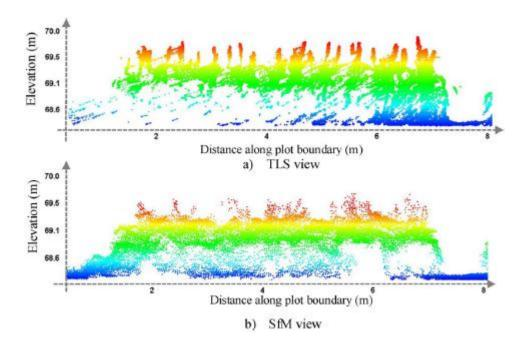
Figure 4: Longitudinal section view of crop point clouds created from TLS and SfM acquired data (Malambo et al. 2018)
