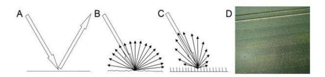
Figure 13: Specular reflectance (A), Lambertian scattering (B), anisotropic asymmetric scattering (C) and an aerial RGB image of a wheat field showing a 'hotspot' resulting from anisotropic reflectance, with the shadow of a UAV visible in the centre (Aasen 2016)
