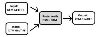
Figure 28: Workflow to compute CSM from DSM and DTM
