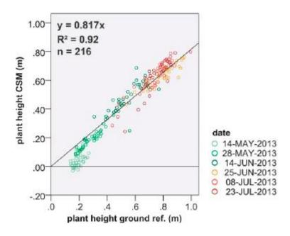
Figure 10: A scatter plot showing correlation between barley plant height as measured from the ground (x axis) against as measured from photogrammetry-derived CSM (y axis) (Bendig et al. 2014)
