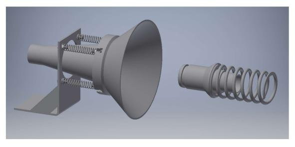
Figure 41: Sprung female mount with male probe and spring
