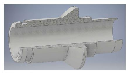
Figure 26: Male component, aka "piston"/probe cross sectional profile
