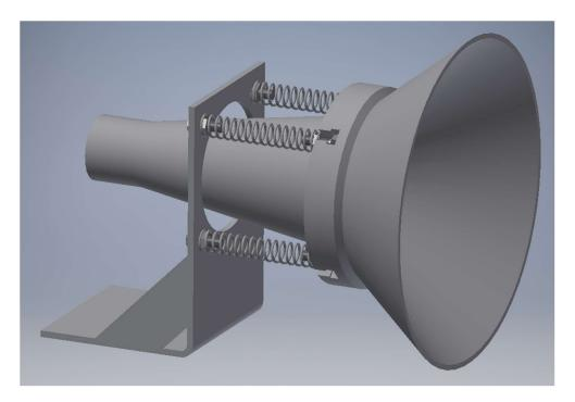
Figure 40: Sprung mounting system for female component
