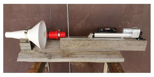
Figure 29: Test rig fully retracted and inline. Female component is white, male is red.
