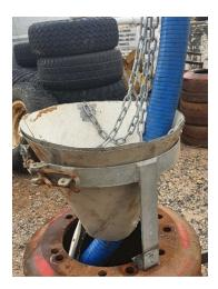
Figure 21: Successful seating at 110mm offset
