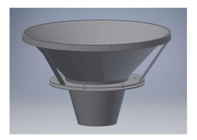
Figure 36: Receiver with flange plates and braced ring
