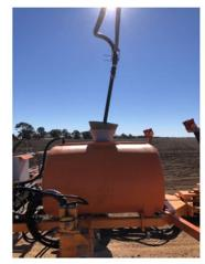
(a) The alignment of the refill hose prior to being (b) The refill hose lowered into the spray tank in the lowered second testing position
