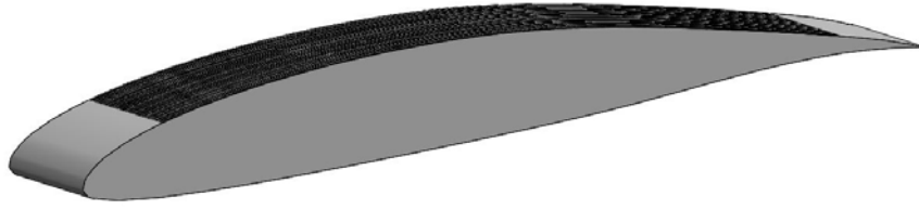
Figure 4.18: S-802 aerofoil section with 50\mu\text{m} - 125\mu\text{m} longitudinal riblets
