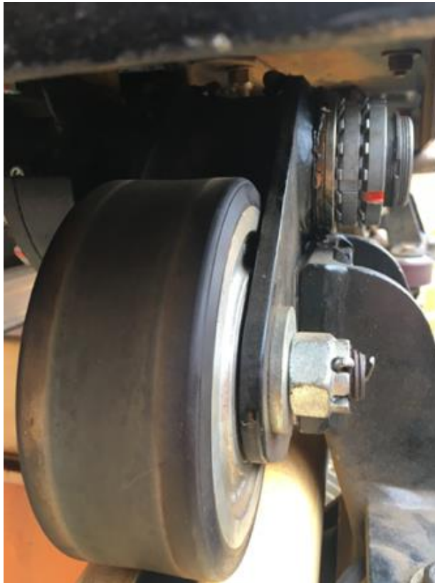
FIGURE 34: TIGHT CLEARANCE BETWEEN ROAD WHEEL AND WHEEL CARRIER
