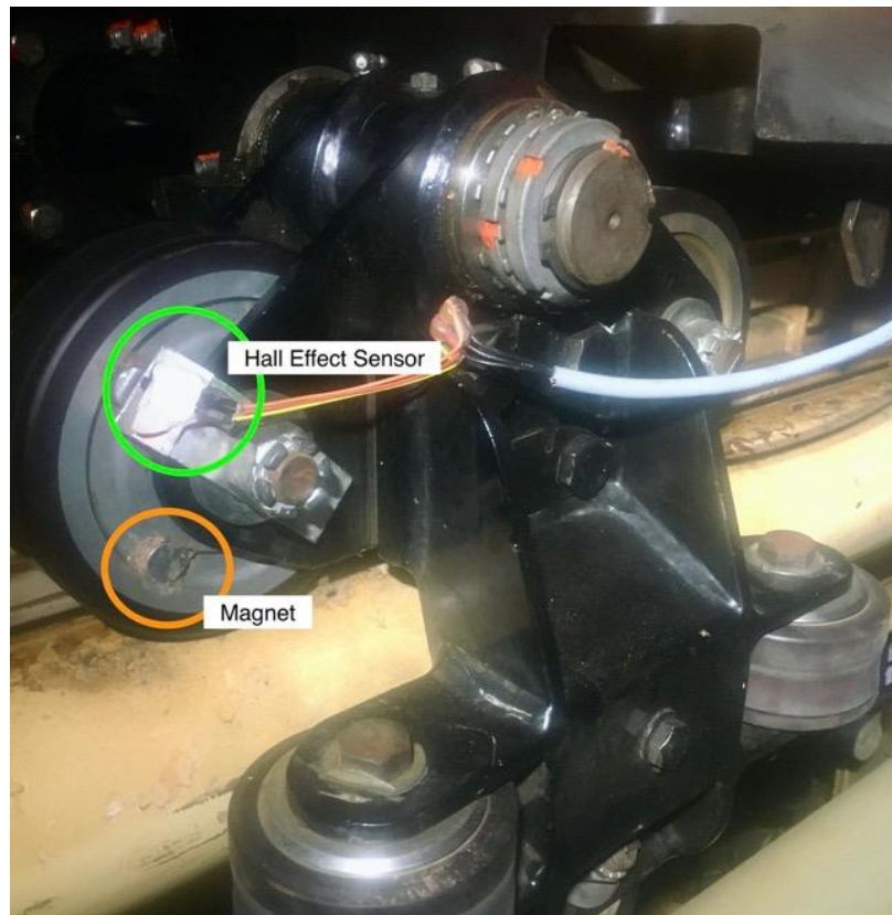
FIGURE 31: HALL EFFECT SENSOR MOUNTED TO WHEEL CARRIER
