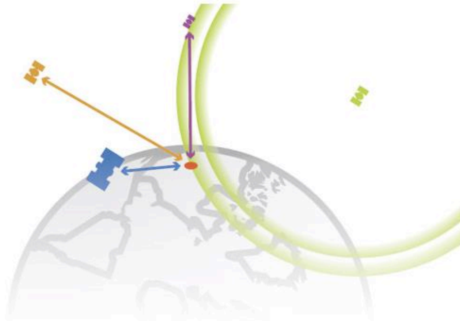
FIGURE 12: FOUR SATELLITES ARE REQUIRED FOR ACCURATE POSITIONING, (SPARKFUN 2020)
