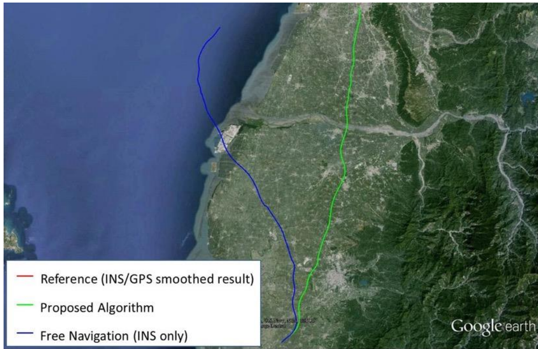
FIGURE 3: THE DELETERIOUS EFFECTS OF SENSOR DRIFT IN NAVIGATION, (KAI-WEI, CHENG-AN & THANH-TRUNG)
