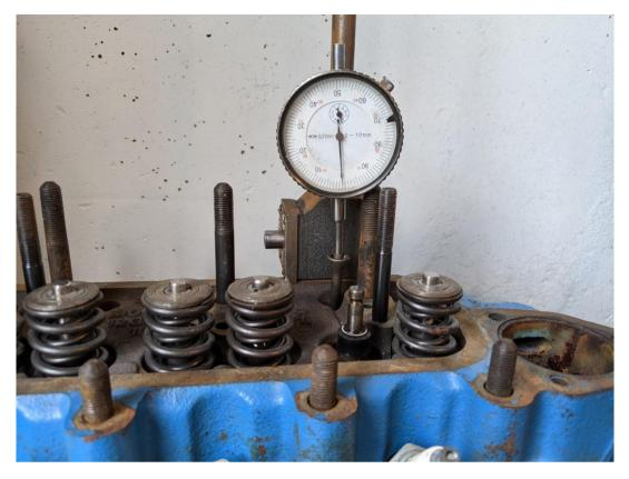
Figure 4.14: Measuring maximum cam lift
