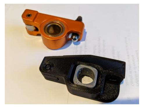
Figure 4.11: Comparison of Harland sharp rocker showing large radius in critical areas
