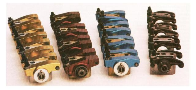
Aftermarket aluminium rockers and standard cast rockers (Calver special tuning-Rocker gear)
