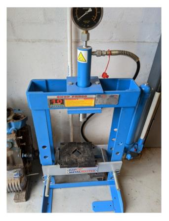
Appendix A.2.2: Hydraulic press for removing valve springs
