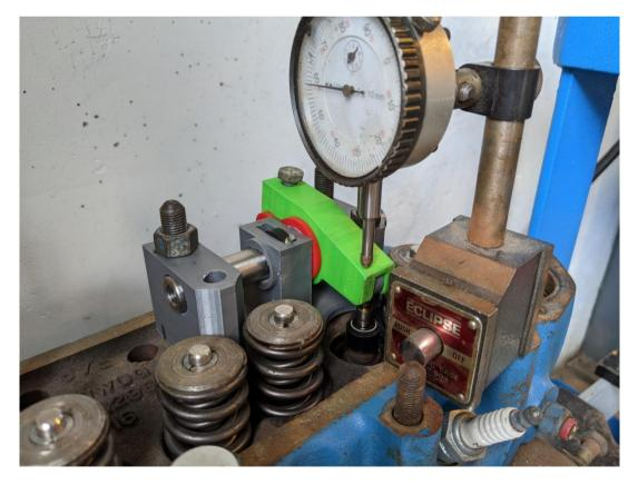
Figure 4.15: Measuring maximum valve lift
