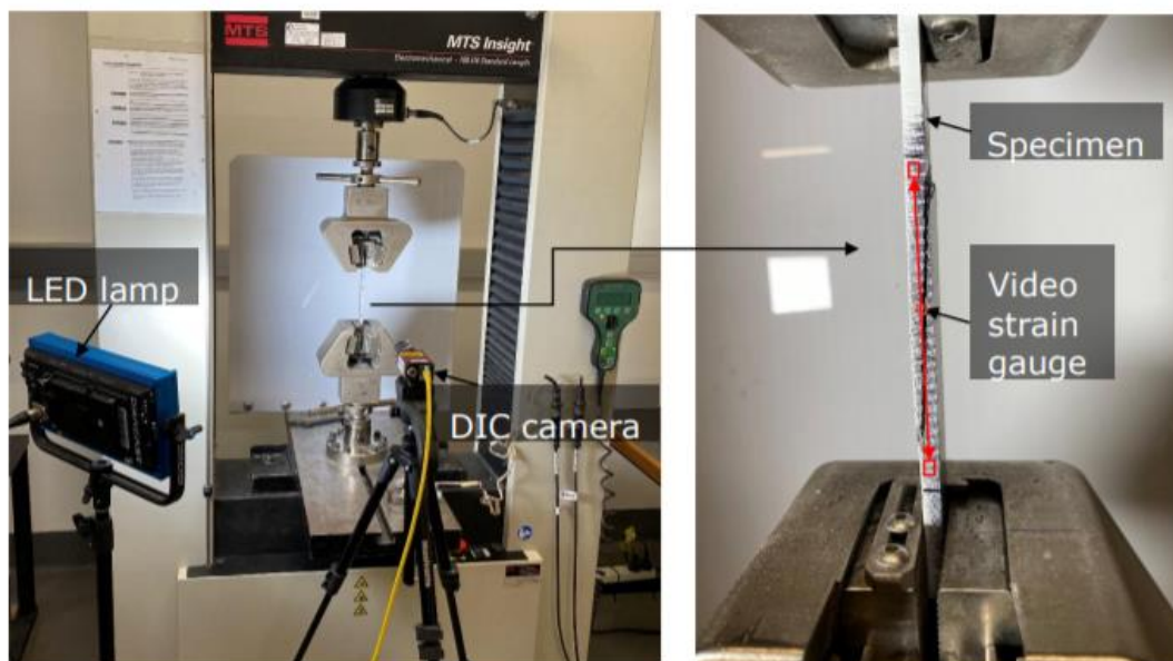
Figure 22: Diagram of tensile testing and DIC rig setup (annotated)
