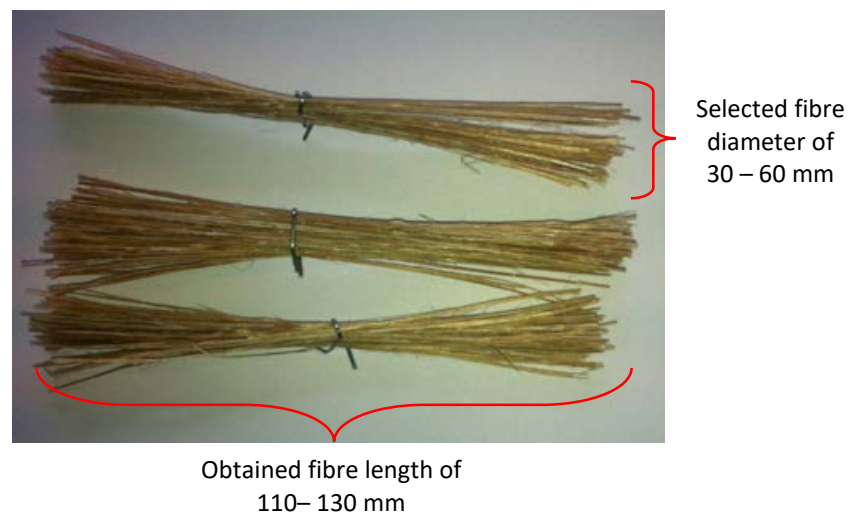
Figure 2. Selected stalked bamboo fibre strips for composite fabrication.
