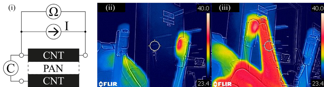
Fig. 4. Experiment: Robot finger shown used in heating mode. (i) test circuit used, (ii) non-heated (left) and heated (right) robot fingers on Baxter's end effector, (iii) robot finger temperatures capable of matching that of human skin.
