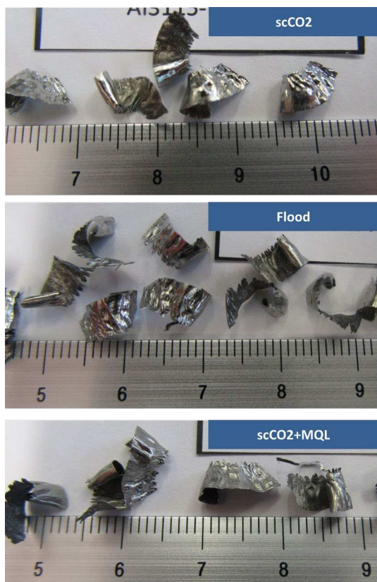
Figure 5 Swarf images collected after cutting trials using scCO 2 , Flood coolant, and scCO 2 + MQL coolant.
