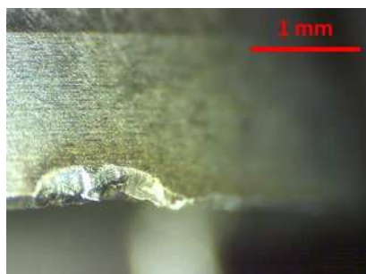
Figure 6 View of the cutting edge at the end of the life trial using scCO 2 + MQL at V c =140m/min
