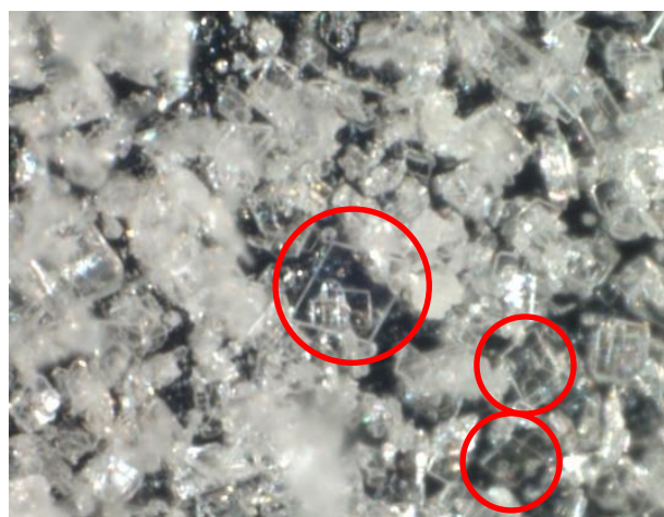
Figure 3: Cocrystal (marked by red circles) obtained from tetramethylurea among other crystals.
