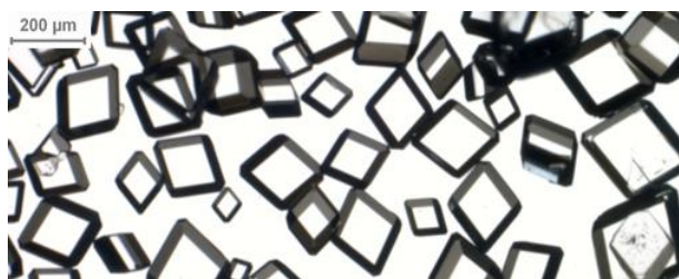
Figure 6: Cocrystal formed in externally-seeded antisolvent crystallisation in ACN at 333 K.
