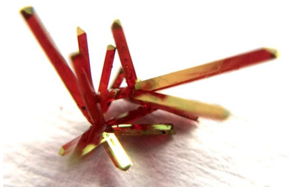
Figure 29: Dichroic crystals of hemiindigo 15 obtained in lengths from 5 to 10 mm. Adapted with permission from [74] . Copyright 2017 American Chemical Society.
