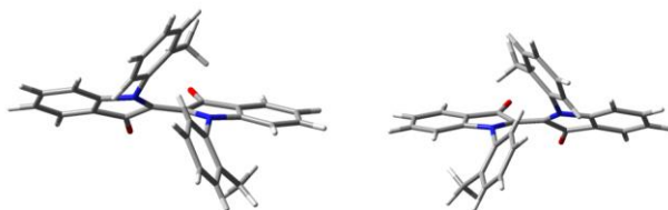
Figure 260: Both hypothetical edge-to-face conformations of indigo 64 that are experimentally stable solely at -60 °C. DFT optimizations at the M05-2x/6-31+G(d) level of theory did not yield local minimum structures.
