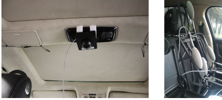
Figure 1: Experimental data gathering. Left: Mean radiant temperature sensor. Right: Upper body of the Flatman thermal manikin.
