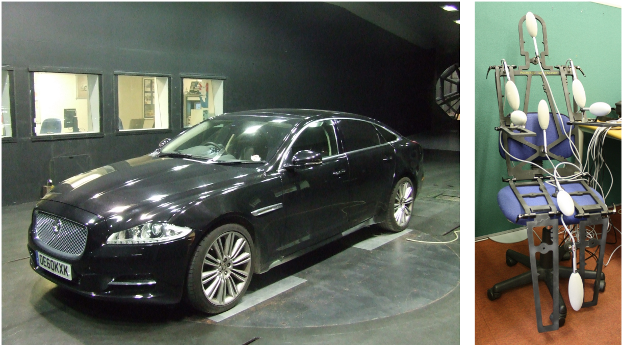
Figure 4.2: Experimental data gathering. Left: Test car. Right: Flatman support manikin with dry heat loss sensors.
