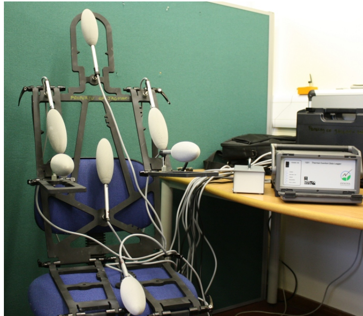
Figure 2.2: The Flatman support manikin, with the associated eight dry heat loss transducers and logger.
