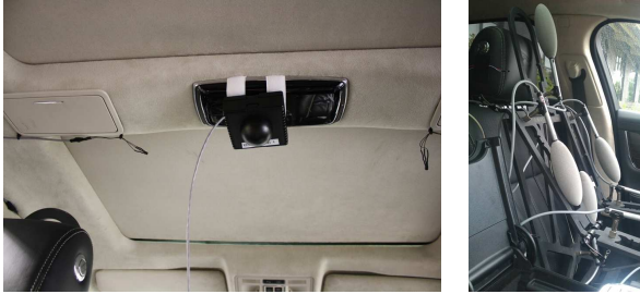
Figure 2: Experimental data gathering. Left: Mean radiant temperature sensor. Right: Upper body of the Flatman thermal manikin.
