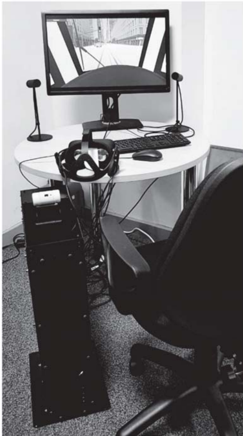
Figure 5. Tram VR simulator including the master tram controller and the Oculus rift head-mounted display (HMD) providing the first-person view of the simulated environment.
