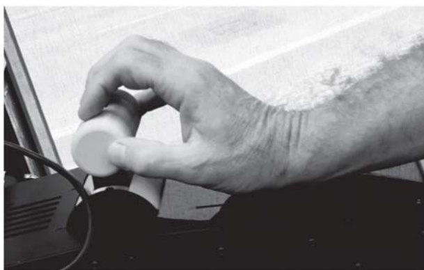
Figure 4. Haptic master controller developed and tested to evaluate its role in improving passenger comfort and safety.
