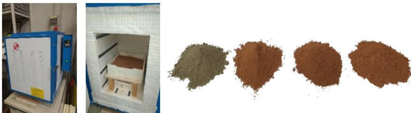
Figure 4. Silt calcination process. Different calcination temperatures change the physical appearance of the silt. From left to right, the images show the uncalcined silt and the silt calcined at 550, 750, and 850 °C.
