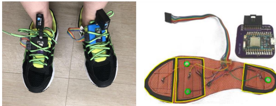
Figure 1.1 Left, subject wearing the DeepSole system. Right, printed circuit board with microcontroller and IMU, and instrumented insole with pressure sensors (yellow outline) and vibration motors (green outline).
