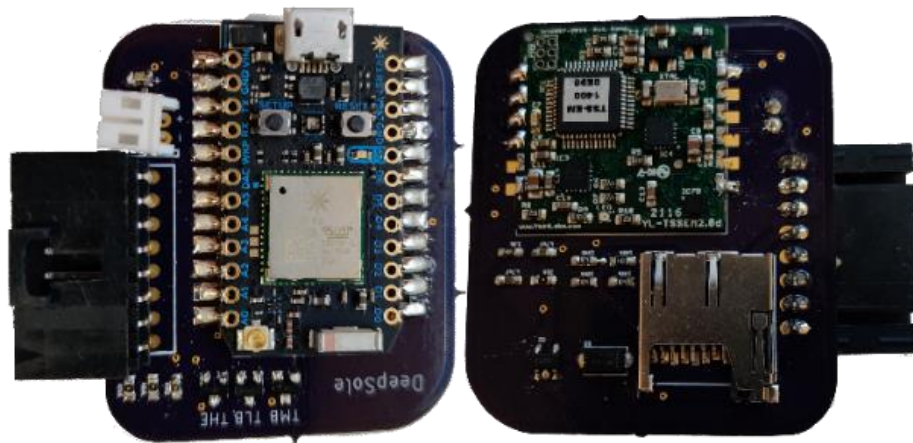
Figure 1.3 DeepSole board. Right is the front of the board; the Particle Photon is the main unit on this side. Left is the back of the board, the micro-SD card and the 3-Space Embedded IMU are visible
