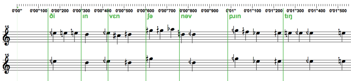
Figure 12: F3 contour data imported with a step size of 50 ms and an amplitude threshold value of 0.0008 (upper staff) and the attack/release points picked by the algorithm (lower staff)
