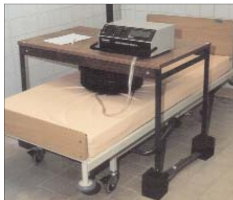
Fig 2. The complete apparatus: indenter, 30kg weight, and the Oxford Pressure Monitor
