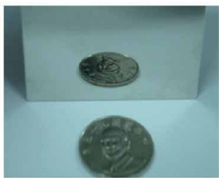
Figure 2. The image of the mirror-like 304 stainless steel substrate after the EP process.
