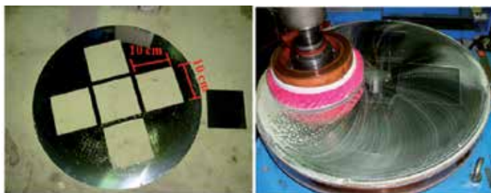
Figure 4. The sample holder and polishing process image of the ECMP system.
