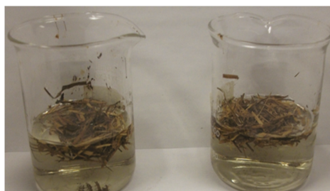
Figure 6. Bitumen samples with charred hay (60 min) added in deionized water (left) and Instant Ocean solution (right) at room temperature (23 °C) and time = 0 h.
