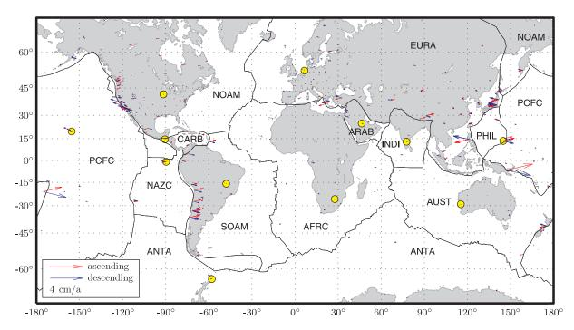
Figure 7.8.: Bias of the baseline error rates  $\delta B'_{\perp} = v_{\perp}$  due to approximation of the ITRF2008 velocities by point velocities computed from NNR-NUVEL-1A, evaluated for Envisat IS2 interferograms at 840 ITRF2008 stations. The arrows are aligned to the horizontal projection of the respective radar line of sight. Mind the enlarged scale with respect to figure 7.3. Numerical values for the twelve encircled stations can be deduced from table 7.1.
