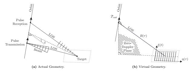
Figure 2.1.: SAR Acquisition Geometry. (a) The platform displaces between transmission and reception of a pulse. The squint angle  $\beta$  is defined in a plane defined by the line of sight (LOS) to the target and back, measured halfway between transmission and reception. (b) The platform maintains its positions between transmission and reception of the pulse (start-stop approximation).
