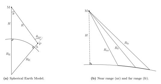
Figure A.1.: Acquisition geometry that is assumed for most numerical simulations. (a) The earth body is approximated by a sphere with a radius of  $R_{\rm E}=6371\,{\rm km}$ . (b) The acquired swath extends from near range  $R_{\rm nr}=\frac{c}{2}\tau_0$  to far range  $R_{\rm fr}=\frac{c}{2}(\tau_0+\frac{n_\eta}{f_{\rm RSR}})$ , where  $n_\eta$  is the number of samples in range. Note that the average range  $R_0$  as defined in eq. (A.5) is *not* bisecting the sensor's field of view.
