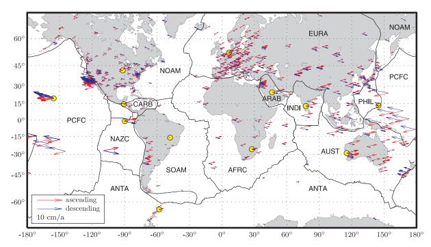
Figure 7.3.: Prediction of baseline error rates  $\delta B'_{\perp} = v_{\perp}$  for Envisat IS2 interferograms from ITRF velocities, evaluated at 840 ITRF2008 stations. The arrows are aligned to the horizontal projection of the respective radar LOS. Numerical values for the twelve encircled stations can be found in table 7.1.
