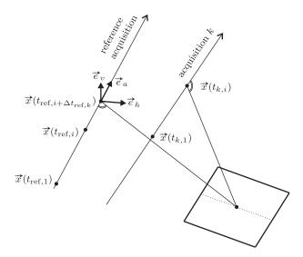
Figure 5.2.: Geometrical relation between the timescales of acquisition k and the reference acquisition that defines the Frenet frame.  $t_{\text{ref},1}$  and  $t_{k,1}$  are the acquisition start times;  $t_{\text{ref},i}$  and  $t_{k,i}$  refer to the respective ith pixel in azimuth.
