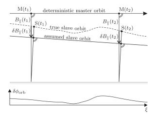
Figure 4.2.: Temporally varying error  $\delta B_{\parallel}(t)$  in the parallel baseline, projected onto a plane defined by the lines of sight of the master acquisition. According to eq. (4.2), the error translates directly into a phase bias  $\delta \phi_{\rm orb}(t)$ .
