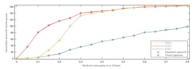
Figure 6.10.: Detectability of simulated unwrapping errors by the dedicated outlier tests  $T_{s,k}$  and  $T_{c,k}$ , respectively. It is displayed in how many of the 163 interferograms a simulated error of a specified magnitude is detected while all other interferograms remain unchanged at the same time.
