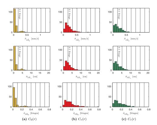
Figure 6.4.: Standard deviations of estimated baseline errors after individual, interferogram-wise estimation as described in section 4.3.1, using different covariance models. The conversion to fringes in the lower row follows eq. (6.6).
