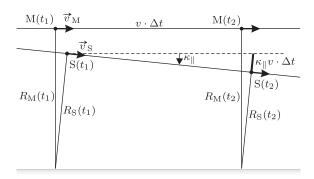
Figure 2.6.: Acquisition geometry with convergent orbits, projected onto a plane defined by the lines of sight of the master. Assuming an orbit convergence angle  $\kappa_{\parallel}$  and constant target ranges for the master, the slave range decreases by a rate of  $\kappa_{\parallel}v$ .
