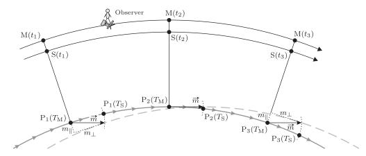
Figure 7.5.: Approximation of a purely horizontal plate motion by the 3D displacement vector  $\vec{m} = (T_S - T_M)\vec{v}$  in P<sub>2</sub> for different azimuth times  $t_i$ . The suggested rotation-free plate motion implies subsidence in P<sub>1</sub> and uplift in P<sub>3</sub>, which does not comply with the actual movement following the curved surface.
