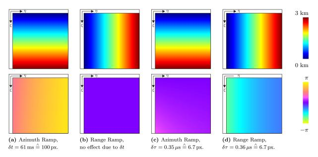
Figure 3.9.: Additional contribution of topography to the patterns induced by timing errors, computed for Envisat IS2 interferograms with  $B_{\parallel}=0\,\mathrm{m}$  and  $B_{\perp}=500\,\mathrm{m}$  and ramp-like generic DEM. The upper row shows the respective DEM and the lower row the corresponding error signals. The latter scale approximately linearly with the terrain slope and nonlinearly with  $B_{\perp}$  and the error itself.
