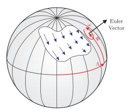
Figure 7.7.: Euler rotation of a tectonic plate about its Euler pole. The plate motion is quantified by the geographic coordinates  $(\Phi, \Lambda)$  of the Euler pole and the angular velocity  $\omega$ . The characterising Euler vector is pointing from the earth's centre to the Euler pole and has the modulus  $\omega$ .
