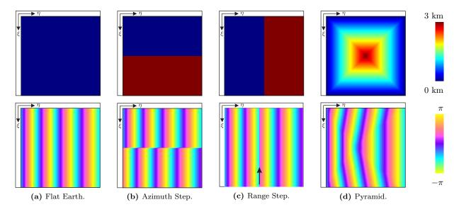
Figure 3.7.: Error patterns in the interferometric phase that are induced by a baseline error of  $4 \delta B_{\perp,2\pi} = 1.05$  m (corresponding to four fringes in range), assuming different generic DEM. The upper row shows the respective DEM and the lower row the corresponding error signals. Note that this effect is independent of the absolute baseline  $B_{\perp}$ .
