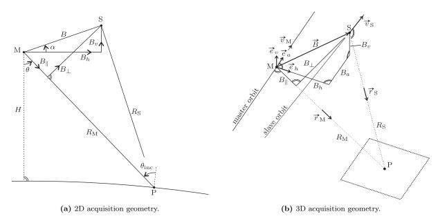
**Figure 3.1.:** InSAR acquisition geometry: A target P on the surface is acquired from point M on the master orbit and point S on the slave orbit. (a) Idealised geometry assuming perfectly parallel orbits, viewed in a plane perpendicular to the flight direction. (b) Actual geometry with convergent orbits.
