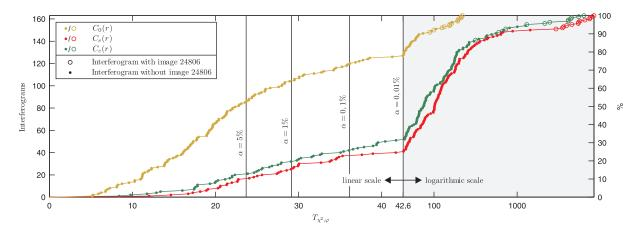
Figure 6.8.: Chi-square goodness-of-fit tests on the interferogram level.  $T_{\chi^2}$  has been computed from the test statistics  $T_{\varphi,i}$  of all  $i=1\dots n_{\varphi}$  pixels of an interferogram. The cumulative distribution of  $T_{\chi^2}$  for all 163 interferograms is visualised by one graph per covariance model. The test fails for a large number of interferograms and any reasonable level of significance  $\alpha$ .
