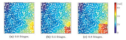
Figure 6.9.: Simulation of unwrapping errors, exemplarily demonstrated on interferogram 14786–15788. All phase observations in a quadratically confined area in the lower right corner are shifted by  $2\pi$ . The extent of the phase shifted area is measured by the fringe equivalent of the induced error signal.
