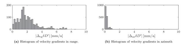
Figure 7.6.: Global evaluation of trends that would result from a correction of the reference frame effect with the translation approach, predicted for full Envisat IS2 frames from one ascending and one descending track at 840 ITRF2008 stations.
