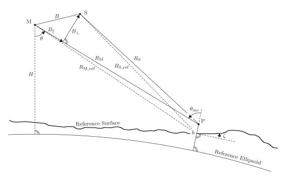
Figure 2.2.: InSAR Acquisition geometry of spaceborne across-track interferometry.
