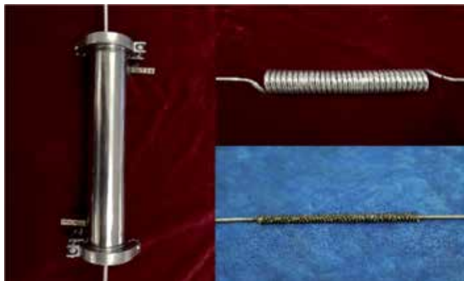
Figure 16. Condenser structure (including two heat dissipation modes).
