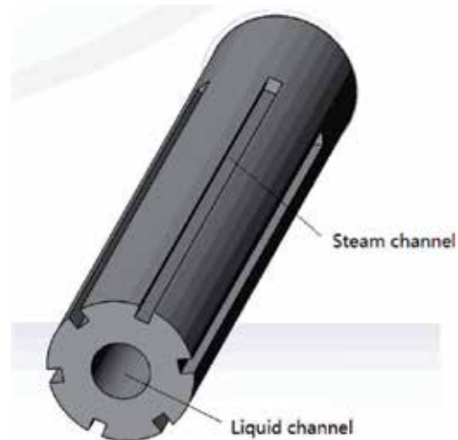
Figure 13. Schematic diagram of capillary core structure.
