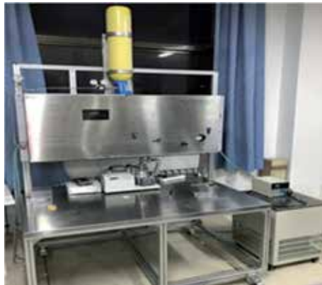
Figure 21. Loop heat pipe vacuum perfusion test bench.
