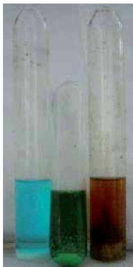
Fig. 13. Digital photograph showing various stages of the hydrothermal reduction of reaction of \text{Cu}_2\text{O} in a sealed tube.
