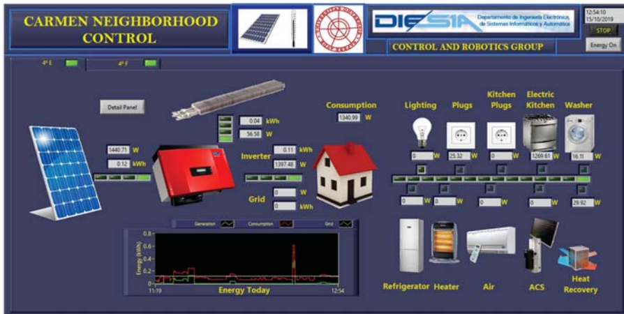
Figure 18. HAS screen. Left: Photovoltaic facility and its production. Right: Electrical circuits of the dwelling.
