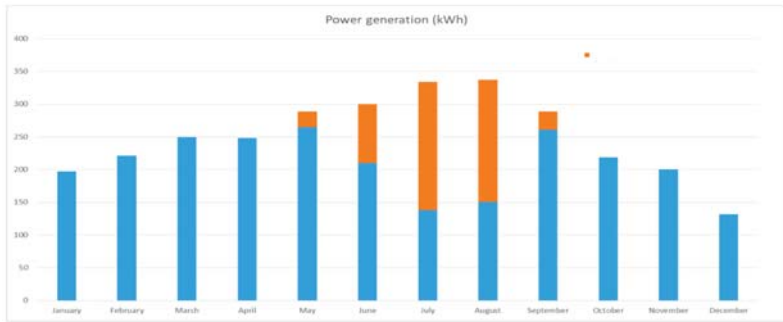
Figure 24. Monthly energy generated (blue + orange) and surplus (orange) in a whole year (2018) after refurbishment.
