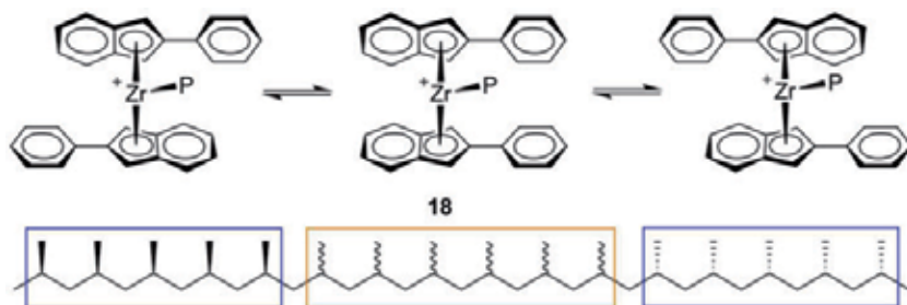
Figure 9. Molecular switching between the two site configurations during polymerization of the unbridged metallocene catalyst.
