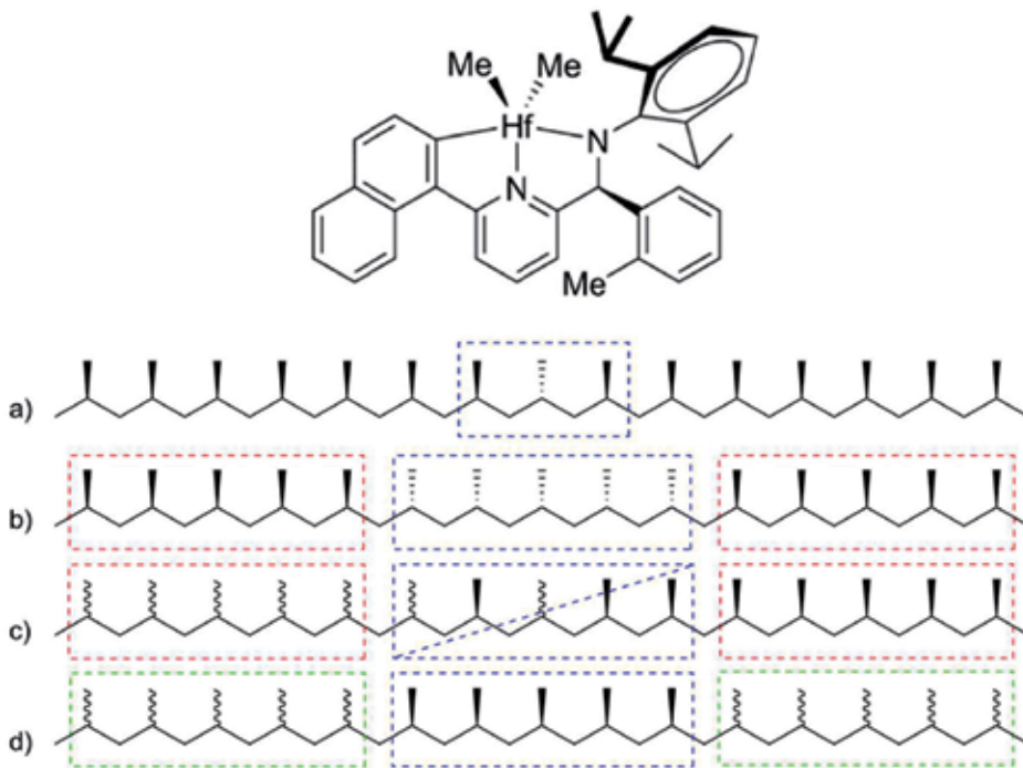
Figure 11. Polypropylene with different stereoisomers: isotactic polypropylene with isolated stereodefects (a), isotactic stereoblock polypropylene (b), gradient (c), and stereoblock polypropylenes (d), which contain hard isotactic and flexible atactic segments [3].
