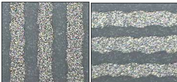
Fig. 12. 100 \mu\text{m} line resolution (after fired) for the silver paste with 10 % thinner weight percentage
