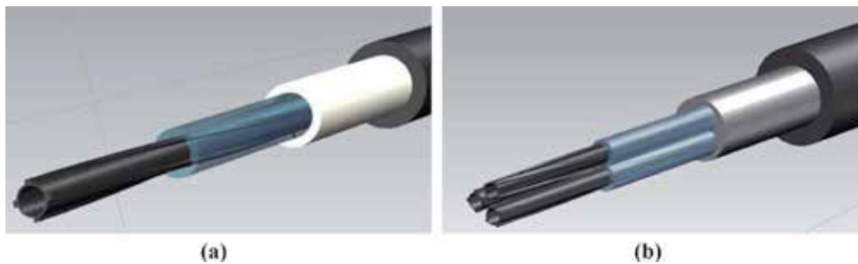
Figure 22. 3-D image of vertical annular channel (a) and three-rod bundle (b) cooled with upward flow of SCW (for other details, see Figure 23 ) [35]: heated rods equipped with four helical ribs.
