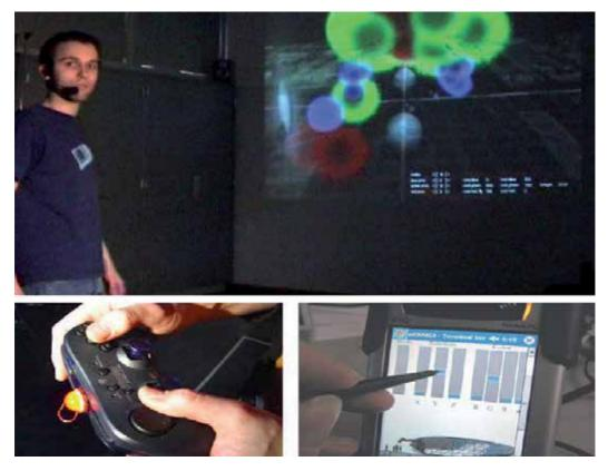
Fig. 3. Protospace: Wireless devices with varying characteristics are available as input devices for implementing specific tasks such as geometrical and behavioral manipulation.
