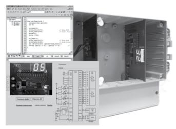
Fig. 10. Remote access laboratory to research microprocessors.
