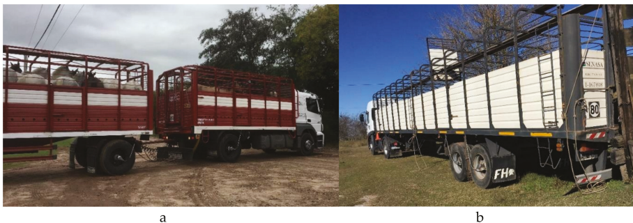
Figure 1. Example of different transport combinations. (a) A truck–trailer: a truck pulling a trailer and (b) A tractor–trailer: a pulling vehicle (without loading space) hauling a trailer through a fifth-wheel coupling.
