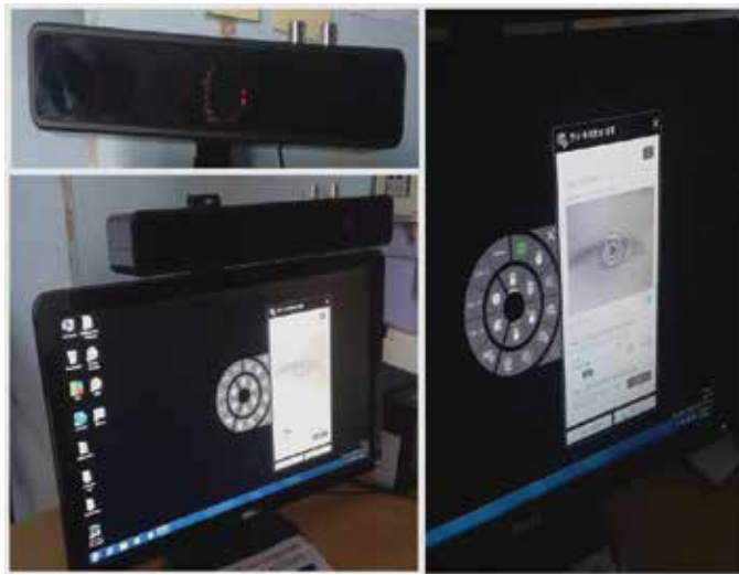
Figure 13. EyeCan+ device fixed to a personal computer.
