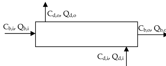
Fig. 1. Schematic description of concentration and flows in dialyzer.
