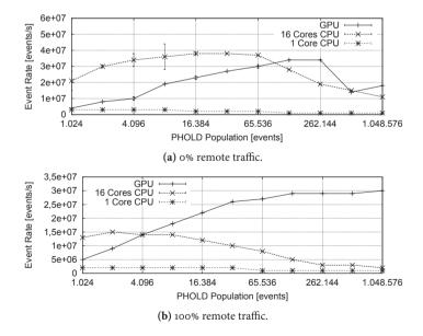
**Figure 10.10:** Event rate of GPU-based simulation of the **PHOLD** model with  $\lambda = 1$ .
