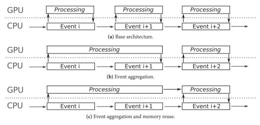
Figure 10.1: Hybrid CPU-GPU-based simulation architectures
