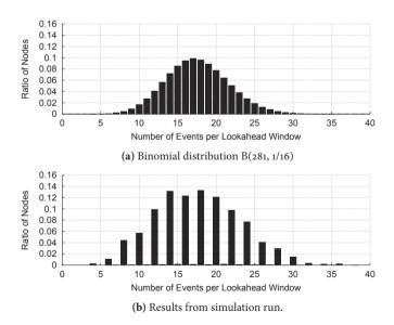
**Figure 5.19:** Expected and observed distribution of the number of events per node of the *hub* category in each lookahead window for a run of the **NMS** model with 16 campus networks, 1 node per LAN, and 1Gbps of hub bandwidth.
