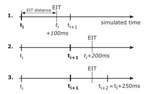
**Figure 9.7:** Chronological sequence of activities performed by  $LP_A$  as an example for waiting times due to synchronization.  $LP_A$  waits for its EIT to advance (1.) before executing further events (2.). At  $t_i$  + 250ms, a remote event arrives from  $LP_B$  (3.).
