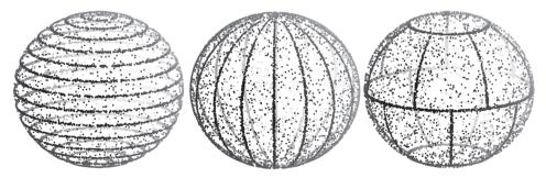
Figure 9.3: In the location-based partitioning scheme, peers are assigned to ranges of latitudes ("discs", left) or longitudes ("slices", middle), or to regions of small diameter and equal size (right) on the earth's surface.
