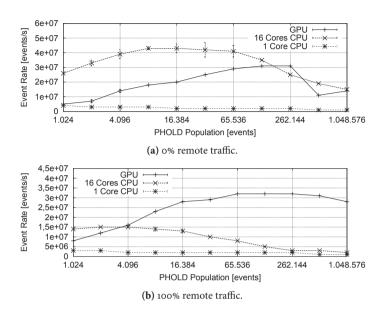
**Figure 10.9:** Event rate of GPU-based simulation of the **PHOLD** model with  $\lambda = 100$ .
