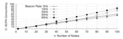
Figure 5.15: Sensitivity analysis of Wireless<sub>A</sub>, varying the number of nodes and the beacon rate.
