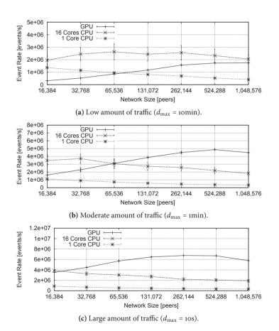
Figure 10.8: Event rate for Kademlia<sub>C</sub> varying the simulator variant, the amount of traffic in the simulated network, and the number of peers.
