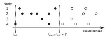
**Figure 5.2:** Synchronization using YAWNS. Events with timestamps  $\leq t_{\text{max}}$  can be processed safely.
