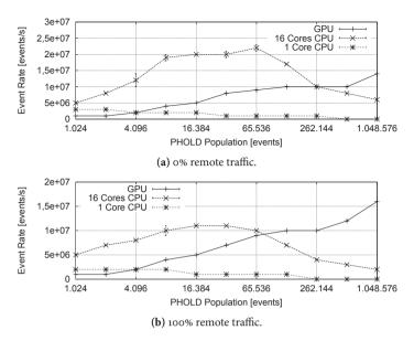
**Figure 10.11:** Event rate of GPU-based simulation of the **PHOLD** model with  $\lambda = 0.01$ .
