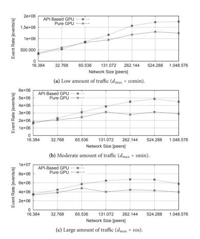
**Figure 10.7:** Event rate for **Kademlia**<sub>C</sub> varying the memory access synchronization method of the GPU-based simulator variant, the amount of traffic in the simulated network, and the number of peers.
