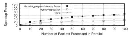
Figure 10.3: Speedup of the proposed hybrid CPU-GPU-based architectures when compared to sequential execution on a CPU.
