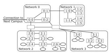
**Figure 5.10:** A campus network in the **NMS** network model. A campus network in the **NMS** network model (Figure adapted from [PR11]).
