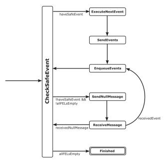
Figure 6.3: Finite state machine description of the LP behavior in SONSim.
